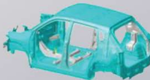
100% galvanization of exposed parts Thin silicon-aluminum coating is applied in hot forming
